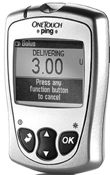
FIGURE 15.3 OneTouch Ping continuous glucose monitor and insulin dispenser. (Courtesy of Animas Corporation.)
