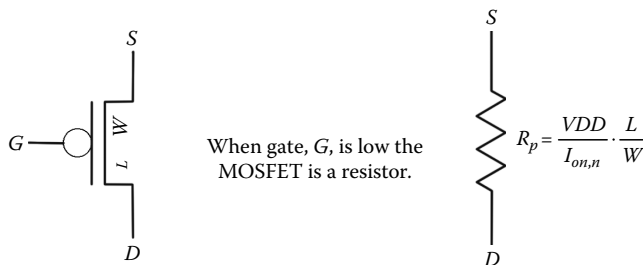
FIGURE 19.5 Digital model of a PMOS device.
